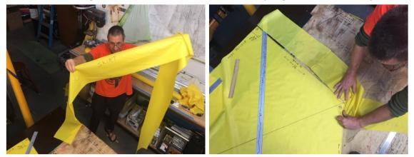
Step 10. Sew the skirt on the bottom (From Point C to B to A and also on other half).
