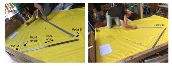
Step 7. Layout Point C. The line from the top to point C is the center "airside", and the two layers will be sewn together here to create the wrap around fly. The line from the top to Point C makes a right angle to Point B (as the triangle Top-B-C is half of the airside of the fly). DRAW A LINE FROM TOP TO POINT C.
