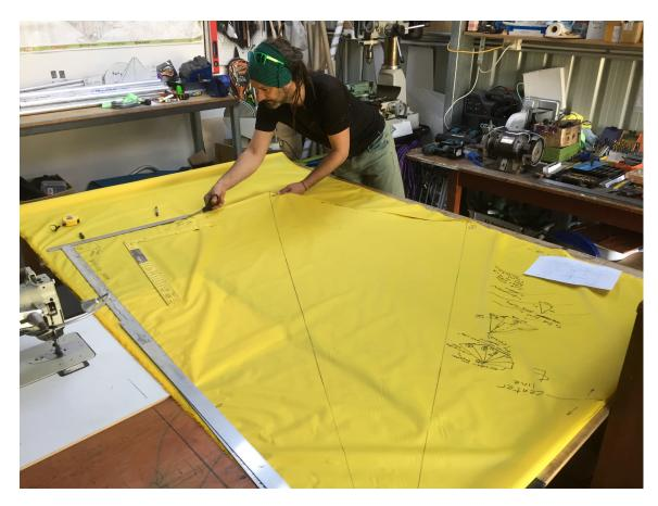
Step 8: Cut out the pattern! Note you are cutting two layers here.
