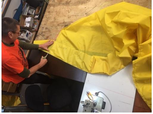
Step 11. Sew the main seam (from TOP to Point C on the two layers). Note on seams: any choice of seams can be used—a simple rollover seam is adequate—all seams will need to be seam sealed for full waterproofing. Hem bottom edge of skirt.
