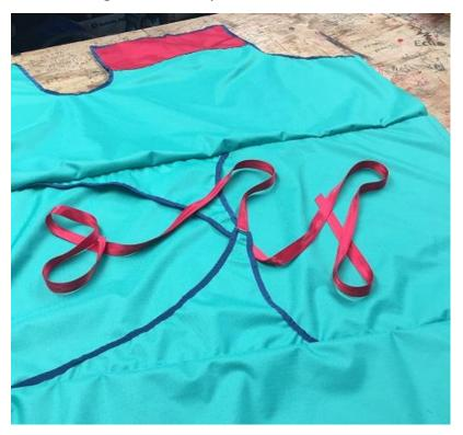
Seamtape all seams and edges except for the wallside and airside fold over.
