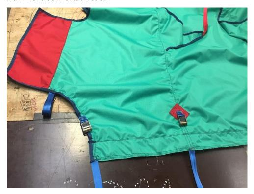
Sew sleeves shut and double stitch. Bartack ends to reinforce. Be precise because there is not much margin for error.
