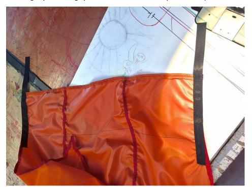
Sew airside sleeve and double stitch. Fold airside strap under to create 3'' loops and bartack.
