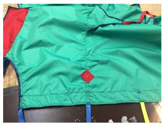
Sew on roller cambuckles, using 3" long pieces of webbing. Two go onto the square patches, the other two on top of the wallside side tensioner webbing 7.5" from wallside. Bartack each.
