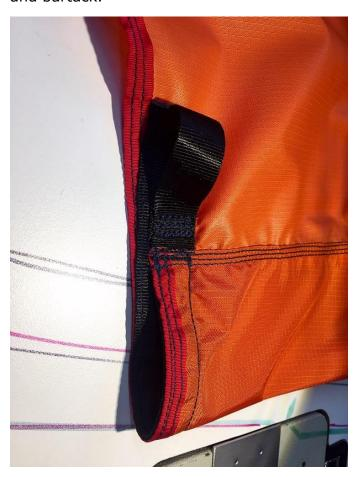
Sew 3" wide webbing onto wrong side wallside, folding in ends and bartacking across the straps. Double stitch on both edges.
