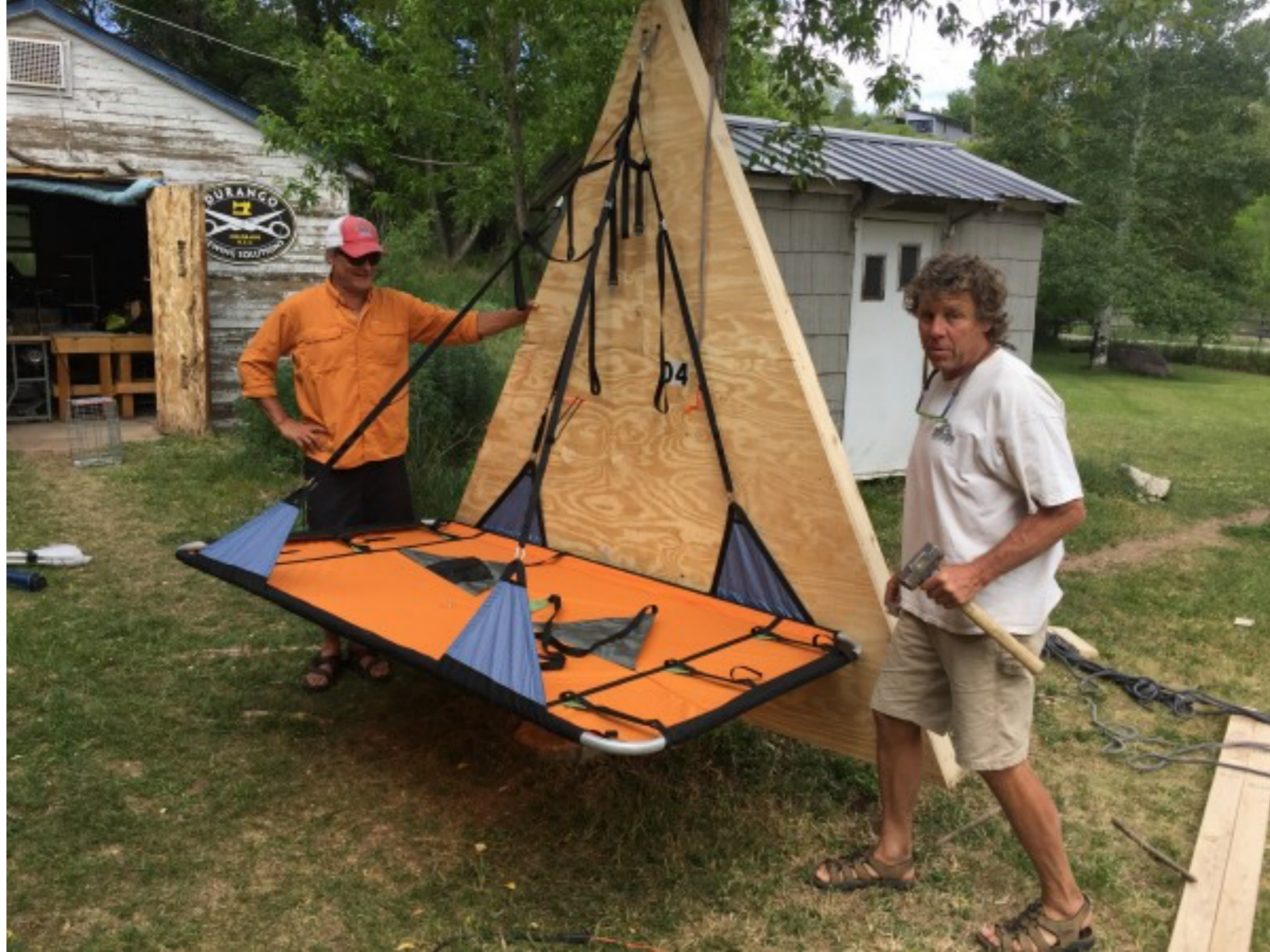
Barr Ward and Steve Quinlan with latest D4 portaledge and new custom variable angle test stand built by Steve. Photo John Middendorf June 3, 2017
