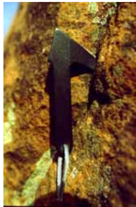
Above: The revolutionary A5 Birdbeak, a thin crack hook, first produced in 1989.
