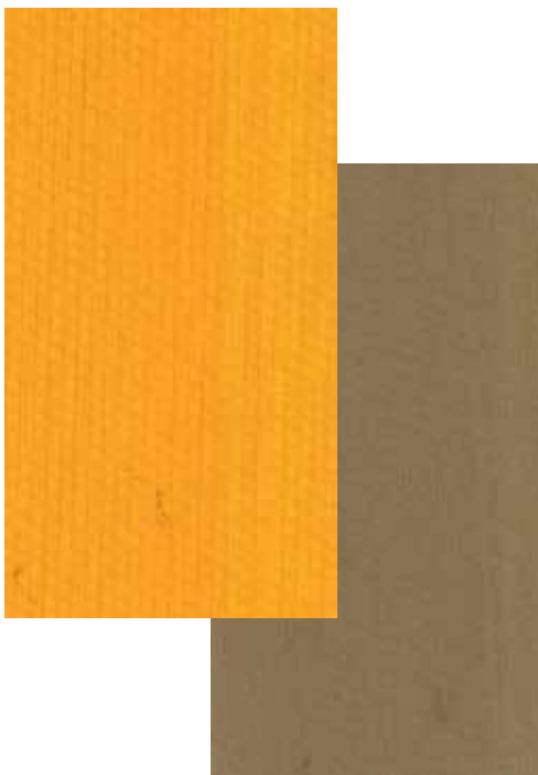
Above: Face and back of a new lightweight waterproof/breathable fabric developed by Middendorf in partnership with the filtration company Tetratek. It is a 3-ply laminate of ripstop/PTFE/tricot. Weight: 3.1 ounces/yd.
