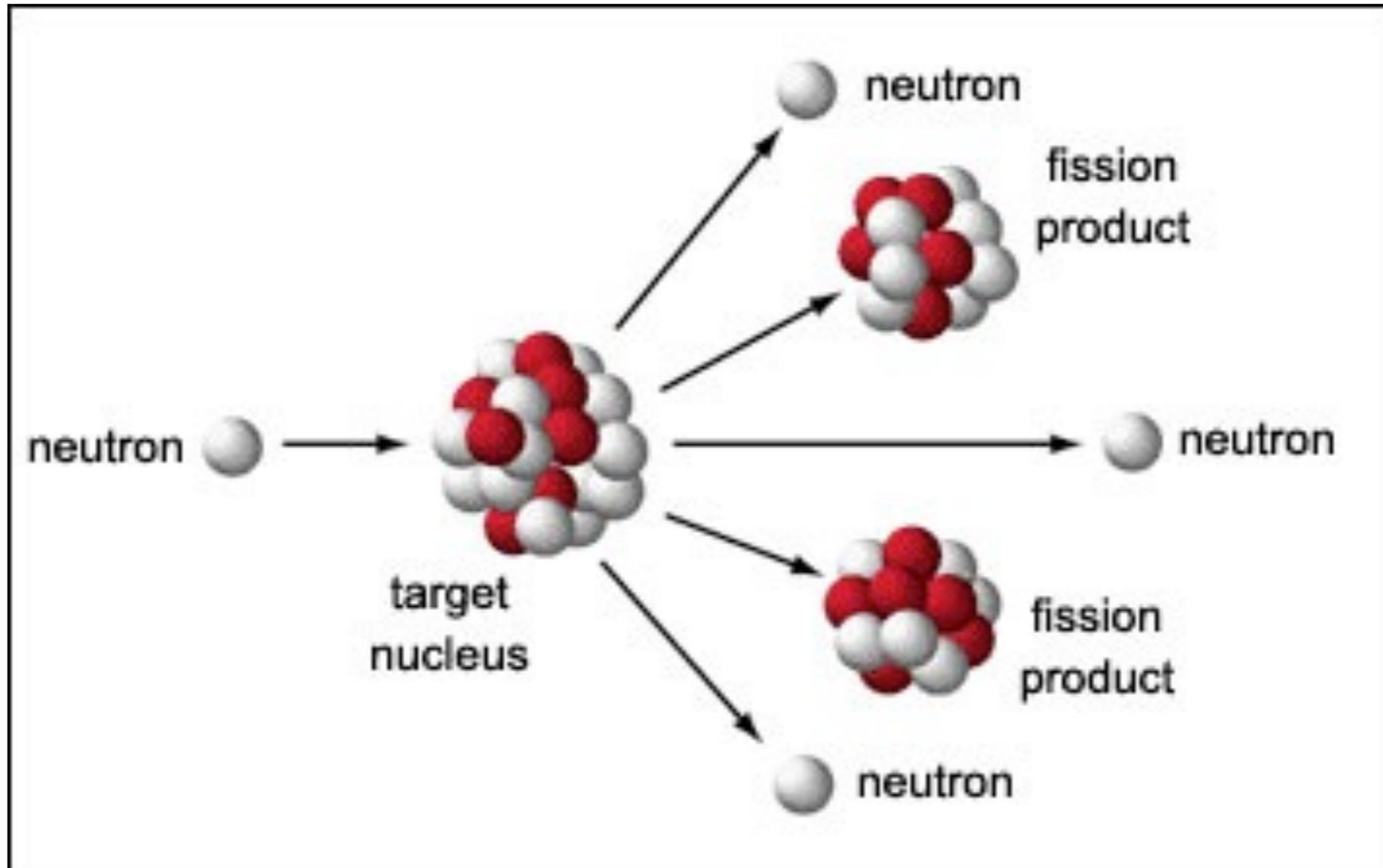
A nuclear reaction involves the splitting of nuclei, usually producing something unstable and releasing neutrons. After a nuclear reaction, a process of emitting radiation (alpha beta and gamma) occurs for it to gain stability.
