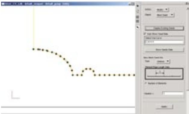
Curve Based mesh seed for 4mm mesh.
