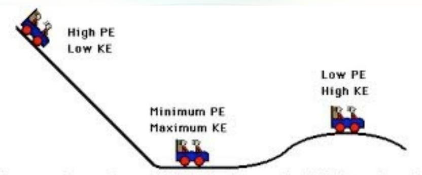
As a coaster car loses height, it gains speed; PE is transformed into KE. As a coaster car gains height it loses speed; KE is transformed into PE. The sum of the KE and PE is a constant.
