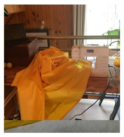
6. Next I sewed the main centre seam of the 'air-side' section. Lacking a waterproof zip, I decided to sew the entire seam closed with about 25cm left open at the very bottom to fit in a zip, giving just enough opening to allow the fly to be closed or opened around the frame but without compromising its waterproof capacity.
